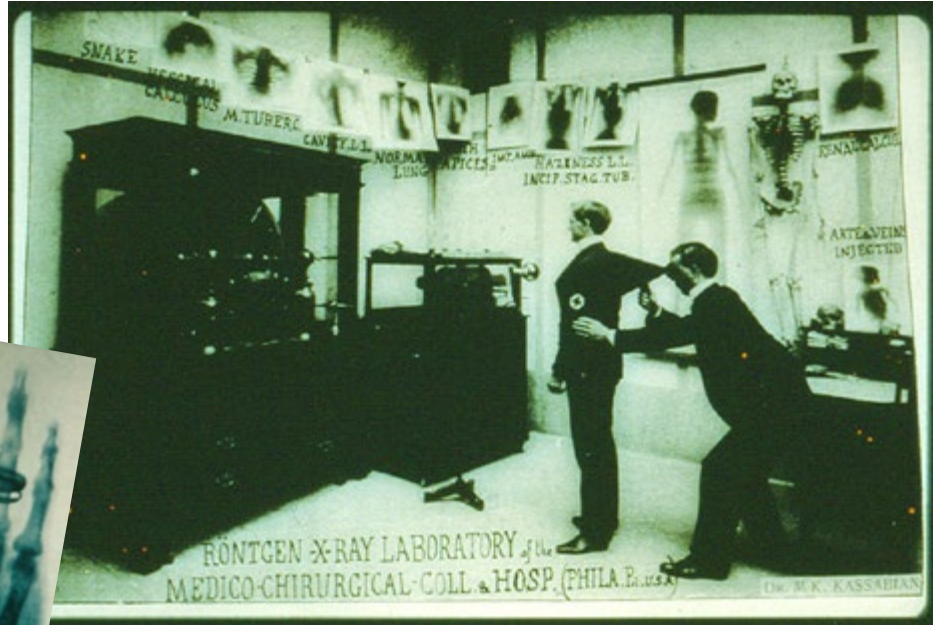
▲ Pictured is Mihran Kassabian at Medico-Chirurgical College and Hospital, Philadelphia, in his radiography laboratory. The large static machine, seen to the left of the image, was used to power X-ray tubes.
